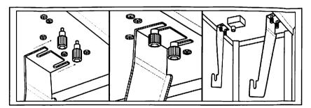
1. Kettle Bracket Assembly: Secure the kettle brackets to the inside top of the popcorn machine. Slide each bracket into position as shown and turn all thumbscrews until secured.
