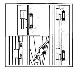
4. Door Assembly: Align the pins on the door hinges with the hinges on the machine.Be certain that the door hinge pins are lined up with the notches on the machine hinges. After the pins are entirely through the machine hinges, turn the door to secure the door in place.
